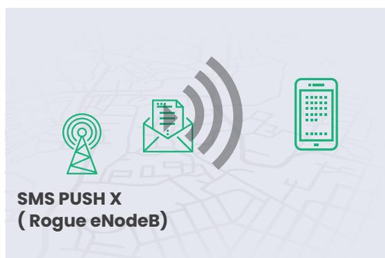
On a 2G network, the attacker can send SMS and even initiate calls with the terminal using any source. 2G network doesn't have mutual authentication in place, thus making it easy to implement MiTM.
